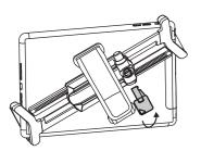
1. Insert the key into the lock slot to unlock the frame.
