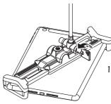
1. Insert the key into the lock button to release the cable.
